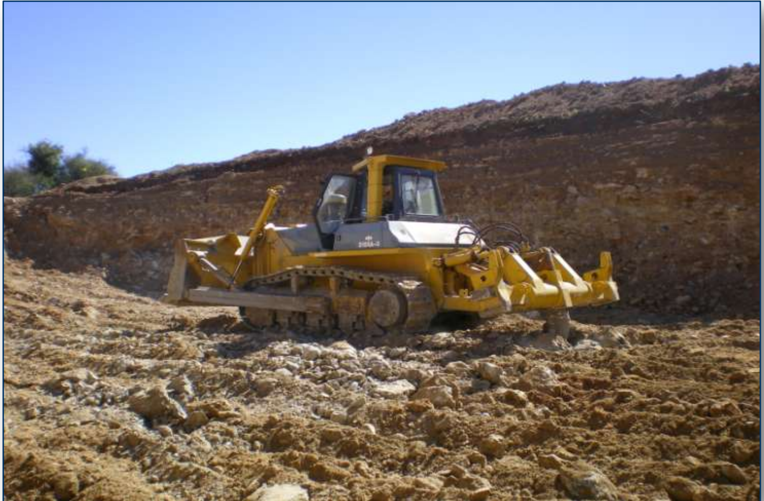
"Ripping & trapping" calcretised gravels during bulk sampling, Harts River - Brussels
