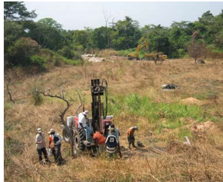
Stripping of overburden and tractor-mounted auger delineating extent of gravels, Dimbi.
