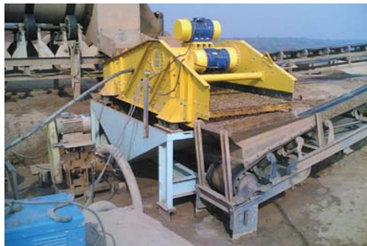
Washed gravels being dewatered, Cassanguidi, Angola.
